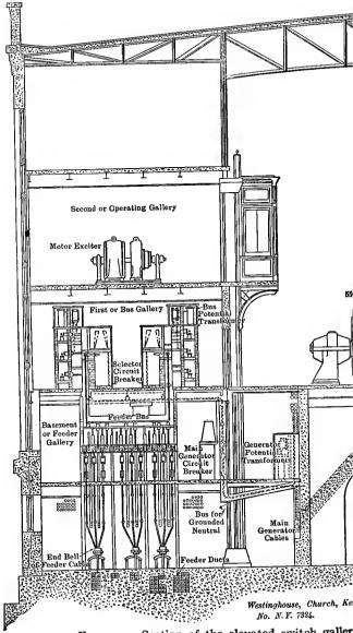
FIG. 120. Section of the elevated switch galler
